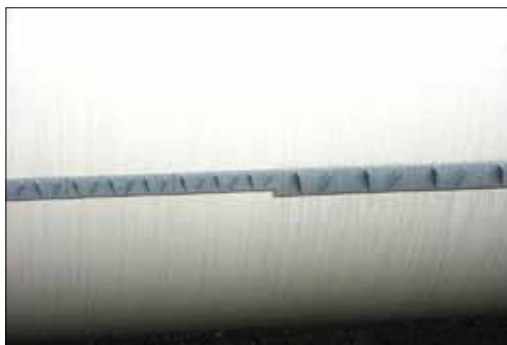
For some time now, “vortex generators” have been used on roller blades to keep wind flowing past the surface of the rotor blade.
